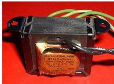
Figure 2.1 Laminated core transformer showing edge of laminations
